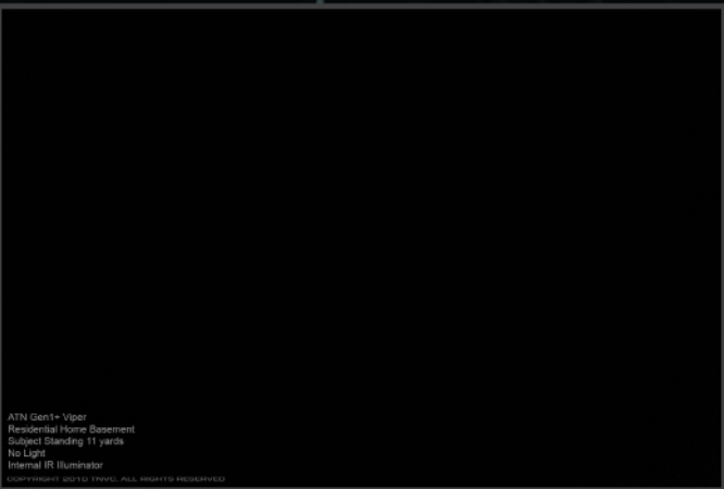
Even with the built-in IR illuminator activated, the Gen1+ tube still cannot produce an image under pitch black conditions.
