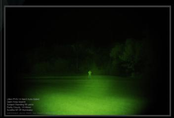
Like the PINNACLE unit, the Litton Gen3 Auto-Gated tube is helped by the introduction of an external IR light source. While the subject is displayed much brighter against the background, the surrounding area is darkened because of the unit's focus on the lighter subject. A darker object is more noticeable in the subject's hands, but it cannot be identified at this distance.
