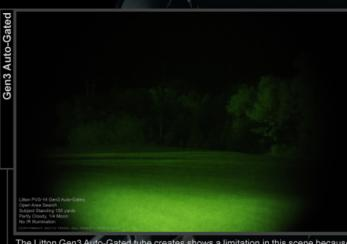
The Litton Gen3 Auto-Gated tube creates shows a limitation in this scene because it is does not produce as bright an image as the PINNACLE unit. The heavy foliage creates a lot of shadow which heavily obscures the subject, making him almost impossible to see. In this situation, an additional IR light source is required.
