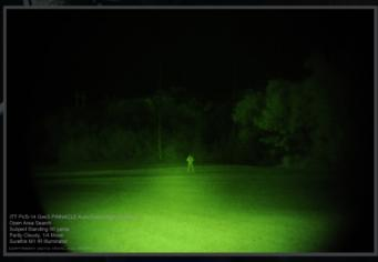
The Addition of the Surefire M1 clearly lights up the subject, causing him to have an almost glowing effect against the surrounding environment. While details become slightly washed out due to the reflection of the IR light, the subject is able to be rapidly acquired at this distance.
