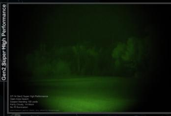
The Gen2 SHP tube produces a full image at this distance. The far tree line is visible, though the subject is partially obscured by the shadows, making it more difficult to detect his presence. It is impossible to determine whether or not a weapon is present. The fine detail seen in the Gen3 tubes is lesser in the Gen2 SHP unit. While it still performs admirably, the overall image is darker and details are grainier.
