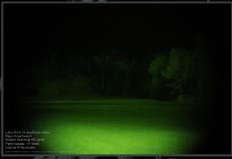
The addition of the built-in IR illuminator does little at this distance. Again, the light gathering limitations of the Gen3 Auto-Gated tube hamper the ability to resolve the subject against the foliage. However, the illuminator does provide a slightly brighter image and the subject does stand out a bit more against the tree line. The definition of his right shoulder, arm, and leg can be seen. However, the details of his posture are unidentifiable.
