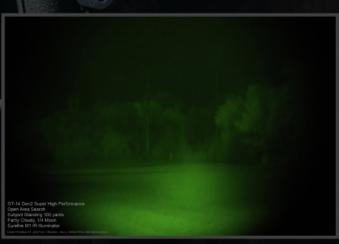
The subject can now be seen against the tree line with the introduction of the Surefire M1. Though resolution is fuzzy, it is possible to detect a man-sized subject at this distance. Details cannot be made out at this distance with this tube, so it is impossible to determine if the subject has a weapon.
