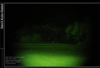
Like the ITT unit, the Litton Gen3 Auto-Gated tube performs well on its own, easily acquiring the subject at 50 yards. The image is slightly darker overall compared to the PINNACLE unit, but enough detail is available to resolve that a single figure is standing in the open with a tree line in the background. Enough contrast is present to decipher the subject's hands in front of his chest, though the presence of a weapon is uncertain.
