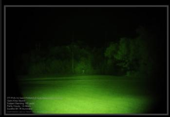
Using the Surefire M1 creates a definite advantage in this search at this distance. The more powerful illuminator helps locate the subject by making him appear much lighter against the foliage background. Detail is better resolved with the subject's arms visibly bent at the elbow. This shows the user that the subject is holding something in his hands.
