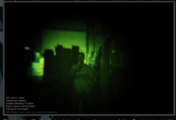
The built-in IR illuminator helps the performance of the Gen1+ tube in this scenario. The subject can be more clearly seen as well as the presence of the weapon. The image is still very dark and details are not readily resolved.
