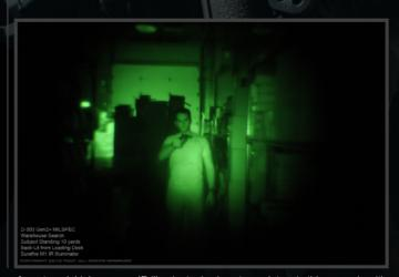
An external, higher-power IR illuminator is almost mandatory in this scenario with the Gen2+ MILSPEC tube. The subject is more clearly defined and the presence of the weapon is quite visible. The added light "pops" the subject from the surrounding environment. Resolution of the surrounding environment drops off quickly and it is still dark, making the detection of additional threats difficult.
