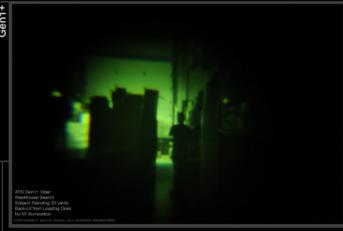
The Gen1+ tube fails to deliver any useable image. The resolution is very poor and the image is completely back-lit, providing no detail of the subject. It is impossible to determine the threat level.
