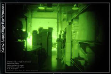
The Gen2 SHP tube performs well in this scenario because of the decent amount of light from the loading dock. The subject is visible, but the weapon is not immediately detected because of less resolution. A second glance will acquire the weapon. Overall, the image shows less-crisp lines and details than the Gen3 units.
