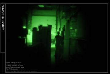
The Gen2+ MILSPEC tube shows serious limitation in this scenario. The subject and foreground are completely silhouetted with no discernable detail. The subject can be acquired, but that is as far as the Gen2+ tube will go. It is impossible to see enough detail to identify the presence of a weapon, so the user has no idea of the threat level.
