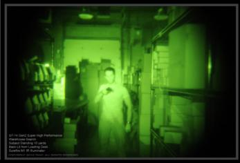
While the image is definitely brighter with the addition of the Surefire M1, it is also noticeably flatter in appearance. This is especially seen in the subject. The Gen2 SHP tube struggles to resolve some detail after the infusion of light. The weapon is still visible, though it is somewhat more blurry.
