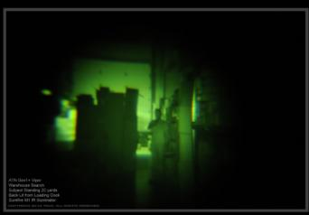
The additional higher-power illuminator is required for any useable image with the Gen1+ tube. However, the lack of resolution is still so apparent, that it is difficult to acquire the weapon.
