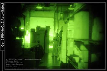
The Gen3 PINNACLE Auto-Gated tube readily acquires the subject and provides a good view of the surrounding environment. Details are resolved and the presence of a weapon is identified.
