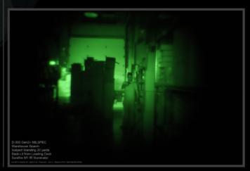
The additional higher-power illuminator is required for any useable image with the Gen2+ image intensifier. Even then, the limited capabilities of this tube produce a dark image. The subject is visible, along with the presence of a weapon. However, the image is too dark to detect any additional threats, limiting the user's situational awareness.
