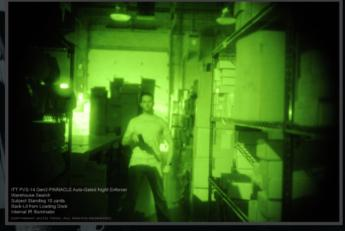
The built-in IR illuminator does not offer much assistance in this scenario. The image is slightly brighter, but sufficient ambient light is already present.
