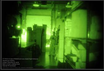
The built-in IR illuminator did not add any value to the image. The back-lit warehouse overpowers the illuminator.
