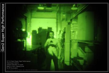
The Gen2 SHP tube provides a good image with good resolution under these conditions. The subject is clearly identified through facial features and the presence of a weapon is certain. The surrounding environment is well resolved.
