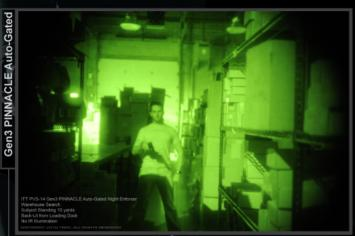
The subject is very clearly seen with facial features identifiable as well as the presence of a weapon. Surrounding details of the environment are visible. The high performance of the PINNACLE tube creates great contrast and allows for extremely high resolution.
