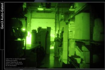
The Gen3 Auto-Gated unit is a bit darker than the PINNACLE tube. While detail is still resolved, the subject appears darker. The weapon is visible.
