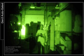
The Gen3 Auto-Gated tube performs well, quickly acquiring the subject and detecting the weapon. Compared to the Gen3 PINNACLE tube, the Litton Auto-Gated unit appears slightly darker. This is more readily seen in the surrounding environment. Note the boxes stacked on the shelves appear to be slightly less resolved. Facial features are still identifiable
