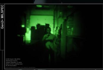
The Gen2+ MILSPEC tube produces a significantly darker image than even the Gen2 SHP. The subject is visible and facial features can be recognized. However, the under-powered tube struggles to provide additional data. For a professional conducting a search, this begins to border on dangerous because the surrounding environment is not nearly light enough to detect additional threats.
