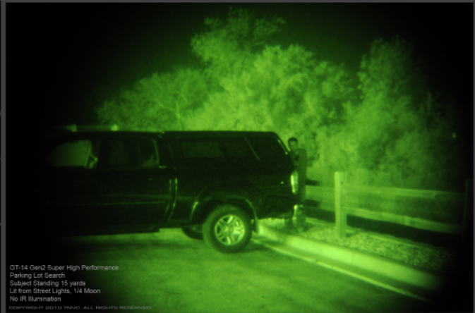
The Gen2 SHP tube does a good job of displaying the image. There is less resolution than with the Gen3 units, but the image is still useable, clearly showing the subject behind the vehicle with a weapon.
