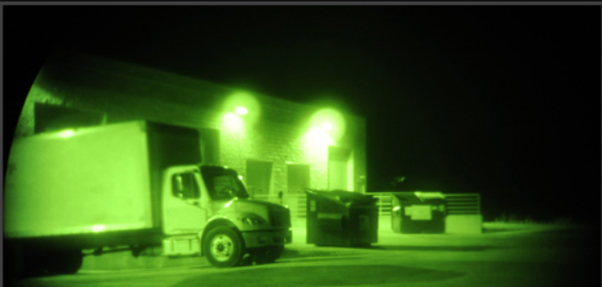
ITT PVS-14 Gen3 PINNACLE Auto-Gated Night Enforcer Loading Dock Search Subject Laying under Truck 50 yards Loading Dock Lights, 1/4 Moon Internal IR Illuminator COPYRIGHT 2010 TRACO. ALL RIGHTS RESERVED
