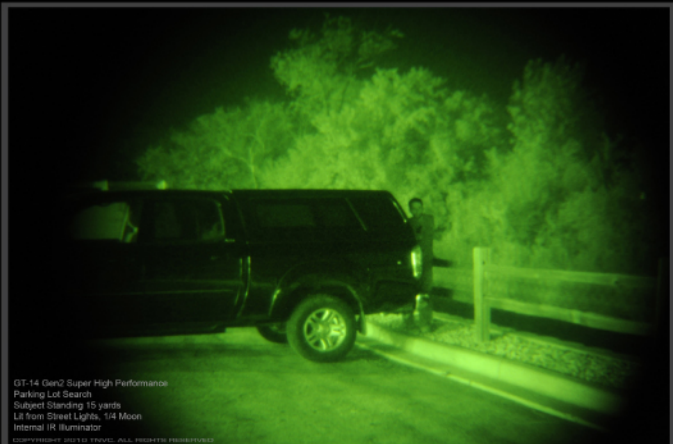
The built-in IR illuminator did not add any value to the image. It is negligibly lighter.
