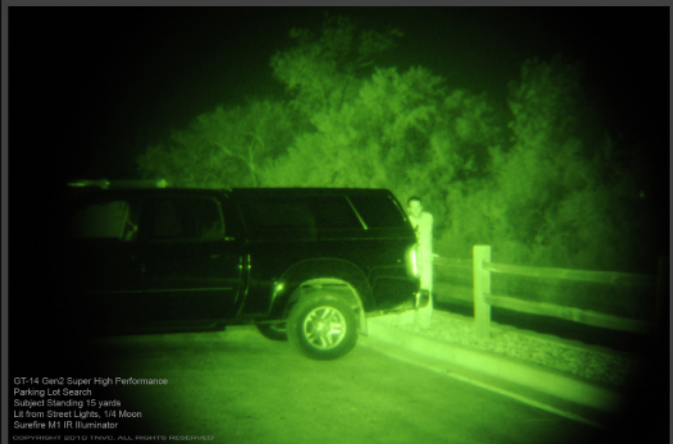
The additional higher-power illuminator brightens the shadows, revealing the subject more. The weapon is clearly seen against the subject's shirt.
