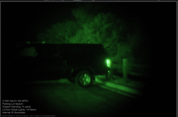
The unit detects a reflection of IR light from the tail light when using the built-in illuminator. This inadvertently draws the user's eye to that location where the subject is partially visible. The weapon is undetected.
