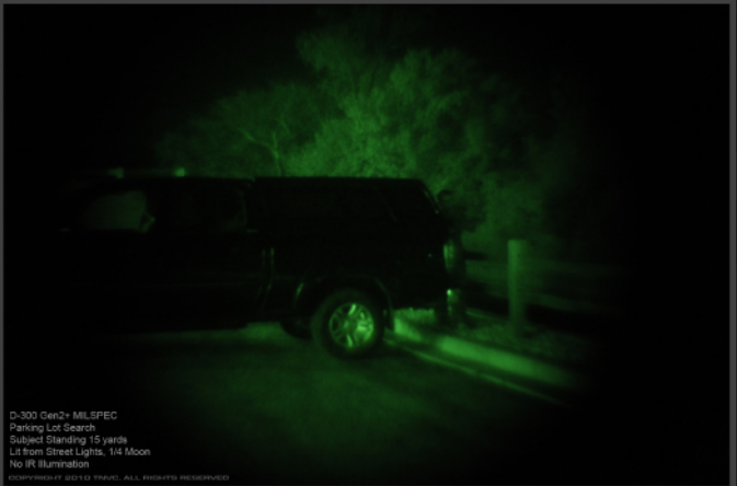
The Gen2+ unit displays a very dark image. Details of the dark vehicle are indistinguishable. The light rims are easily seen. The subject is almost completely obscured behind the vehicle, making it almost impossible to acquire him.
