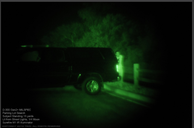
The additional higher-power illuminator is required to observe the subject and see the presence of a weapon. Other details are still much obscured because of the relatively poor light-gathering abilities of the Gen2+ tube.
