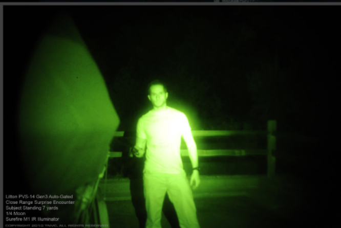
The Surefire M1 focuses the IR light on the subject, creating a hot spot on the torso. The image is not as bright as the PINNACLE, which causes a little less recognition of the hands. The cell phone is harder to read compared to the pistol.
