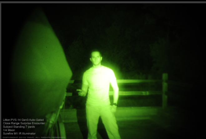
The Surefire M1 focuses the IR light on the subject, creating a hot spot on the torso. The image is not as bright as the PINNACLE, which causes a little less recognition of the hands. The cell phone is harder to read compared to the pistol.
