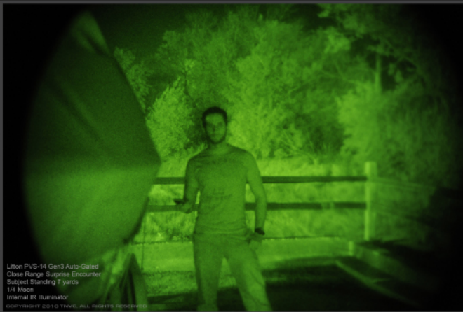
Again, the built-in IR illuminator does little more than flatten some of the contrast in the images. The subject's eyes reflect the IR light. The objects in his hands are easily identified.
