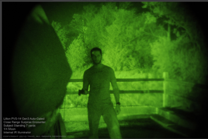
Again, the built-in IR illuminator does little more than flatten some of the contrast in the images. The subject's eyes reflect the IR light. The objects in his hands are easily identified.
