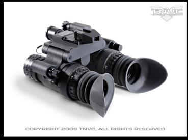
With that said, we are thoroughly impressed with Night Vision Depot's BNVD-G. The BNVD-G uses dual ITT Gen 3 (US) PINNACLE gated tubes. The tubes are fully collimated and feature independent gain control. The technical specs are available on Night Vision Depot's website (www.nvdepot.com), so I will not belabor the details here. Instead, let's discuss the practical applications and features.
