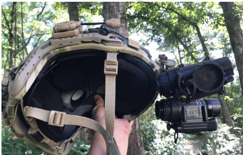
Figure 6. Individual TNV/PVS-14 MNVDs mounted to Noise Fighters Panobridge, TNVC File Photograph
