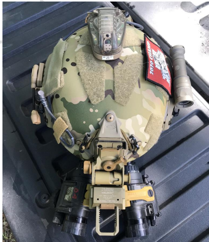
Figure 5. Noise Fighters Panobridge set at approximately 55-60° FOV, TNVC File Photograph
